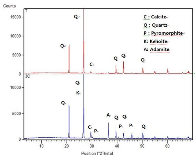
Fig. 2 X-ray diffraction analysis of raw and stabilized sludge with PMW amendments
