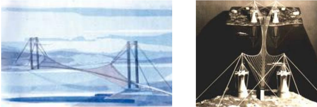
Fig. 1 Nervi's solution with inclined cables
